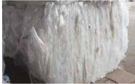
Foils compressed into bales
