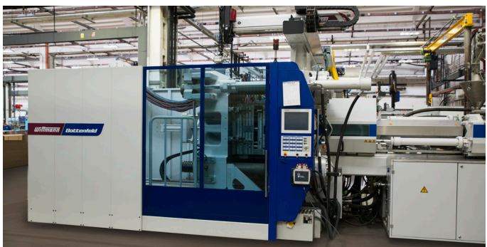
BATTENFELD, Locking force 6 000 – 8 000 kN
